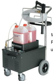
IdroFoamRinse is an innovative machine, electrically powered, allowing to spray foam and rinse continuously. The water used for foaming and rinsing is directly taken from the water network, therefore the machine has an unlimited autonomy. Pure chemical is contained in its separate tank, and it is automatically used by the machine in a controlled quantity.
